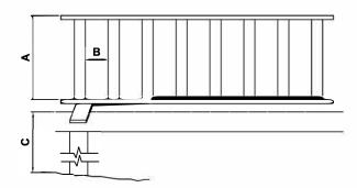
IF "C" IS 2' - 6' (600mm - 1800mm) "A" MUST BE A MINIMUM OF 36" (900mm) IF "C" IS 6' (1800 OR GREATER) "A" MUST BE MINIMUM OF 42" (1.07m)
