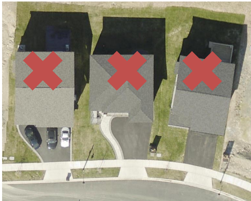
Figure 11-5 - Examples of Unacceptable Driveways
